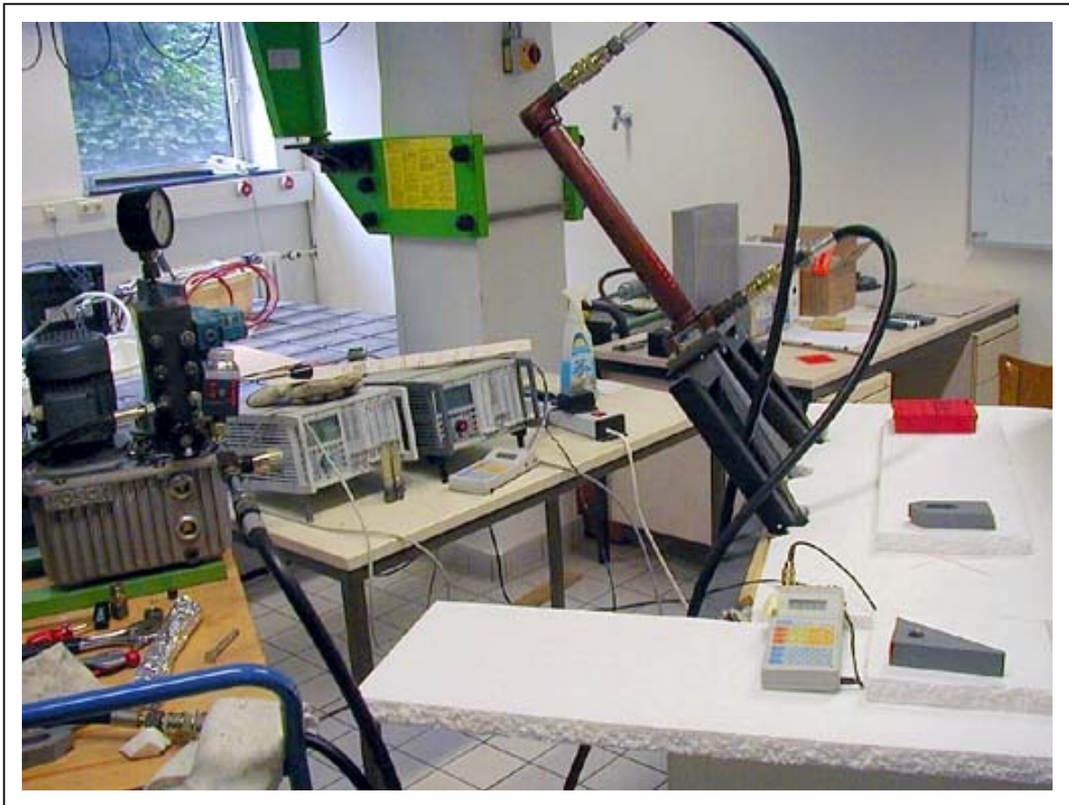
The photo shows the situation during the tension test, in front the temperature display for the measuring point on the suction cup.
